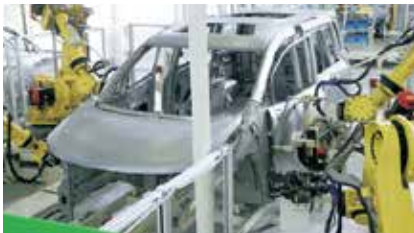
Automatic assembly of doors with the aid of robots (Body Shop)
