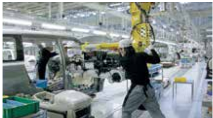
Assembly of heavy parts using assisting devices (Assembly Shop)
