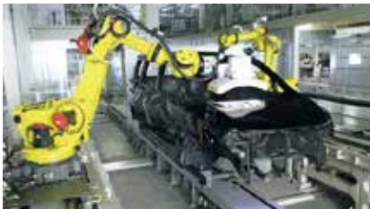
Quality checks on the painted surfaces by robots (Painting Shop)
