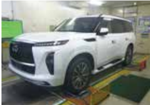
4 wheel shaking machine during the final inspection process
