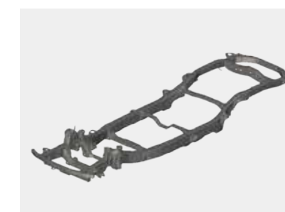
A CAE analysis image used to consider frame designs. We will further deepen the manufacturing technologies unique to Nissan Shatai, such as next generation frame-vehicles, etc.
