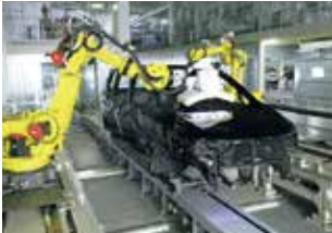
Quality checks on the painted surfaces by robots (Painting Shop)
