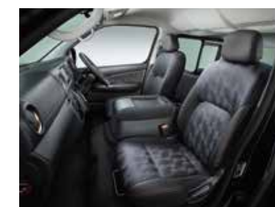
A seat equipped with spinal support in the Caravan which enables the driver to avoid tiredness even on a long drive. It was adopted for the first time in commercial vehicles
