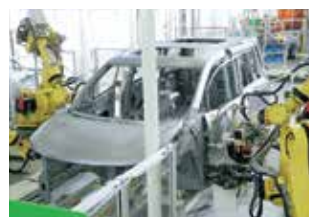
Automatic assembly of doors with the aid of robots (Body Shop)
