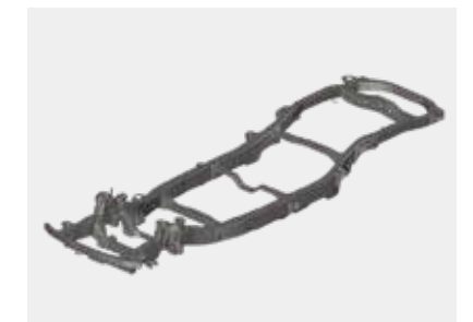
A CAE analysis image used to consider frame designs. We will further deepen the manufacturing technologies unique to Nissan Shatai, such as next generation frame-vehicles, etc.
