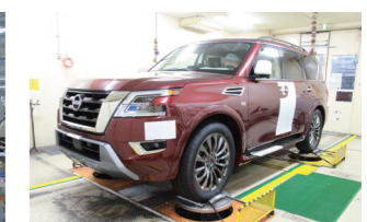
4 wheel shaking machine during the final inspection process
