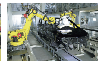
Quality checks on the painted surfaces by robots (Painting Shop)
