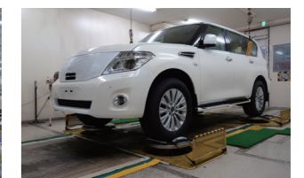
4 wheel shaking machine during the final inspection process
