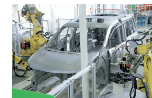
Automatic assembly of doors with the aid of robots (Body Shop)
