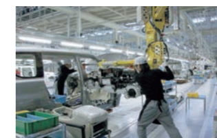
Assembly of heavy parts using assisting devices (Assembly Shop)
