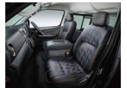
A seat equipped with spinal support in the Caravan which enables the driver to avoid tiredness even on a long drive. It was adopted for the first time in commercial vehicles
