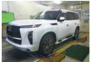
4 wheel shaking machine during the final inspection process
